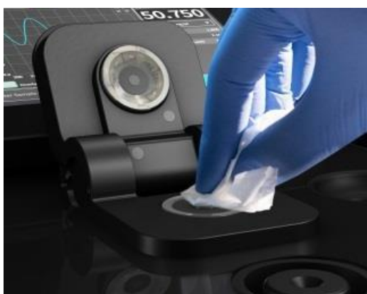
Figure 40. Cleaning the sample illumination window with a laboratory wipe (Reused from: NanoPhotometer NP80/N60/N50/C40 User manual).
