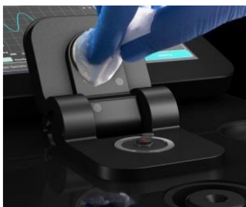
Figure 40. Cleaning the sample illumination window with a laboratory wipe (Reused from: NanoPhotometer NP80/N60/N50/C40 User manual).
