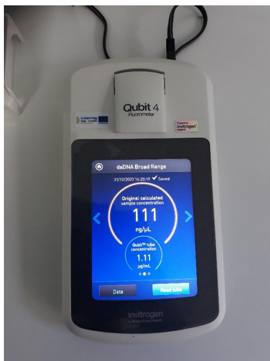
Figure 31. Qubit fluorometer: screen showing the result of the DNA concentration reading (Author: L. Žuvić).
