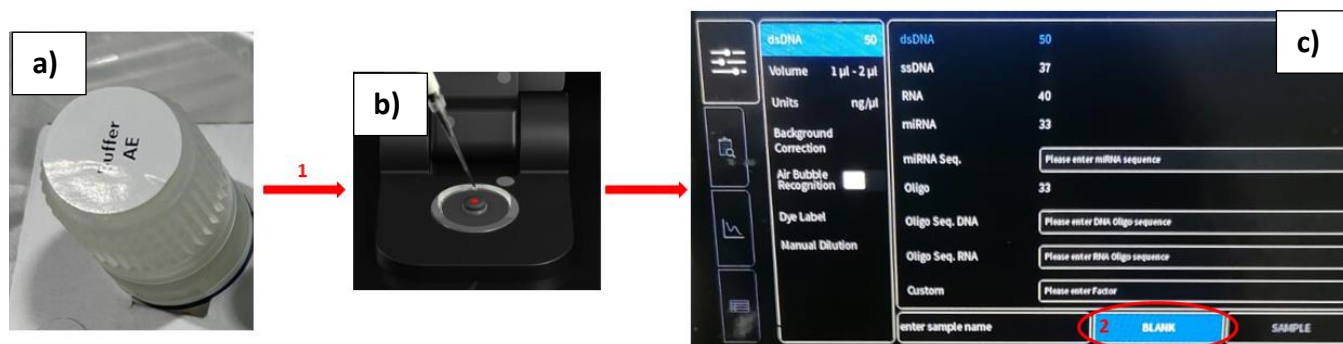
Figure 38. AE buffer (a), Implen NanoPhotometer N50: Application of the AE buffer to sample illumination window (b), screen for calibration and settings (c) (Author: L. Žuvić).
